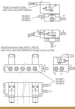
**Ordering Example:** To activate and control 5 pcs. Series PKS-300 simultaneously
